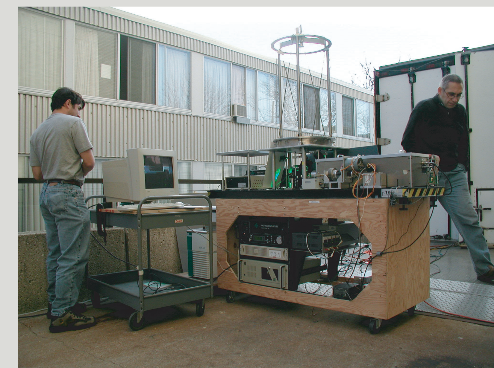
The Arctic HSRL during first alignment and focusing tests which produced the lidar cross section displayed above. The system was mounted on a temporary table and the detectors wired to the our existing HSRL to allow data acquisition before the new data system was available. The system was operated as a standard lidar without the iodine filter for these tests.
