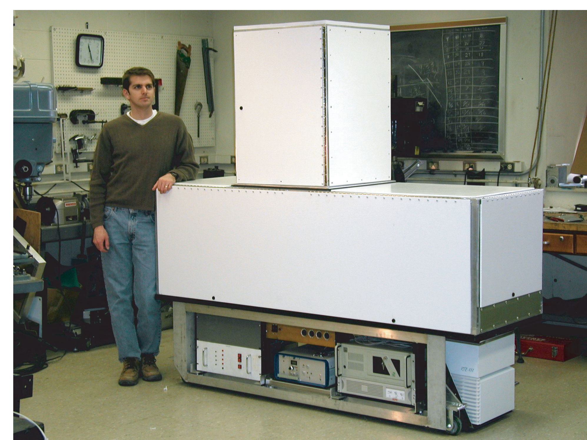
The lidar mounted in it's temperature controlled housing
