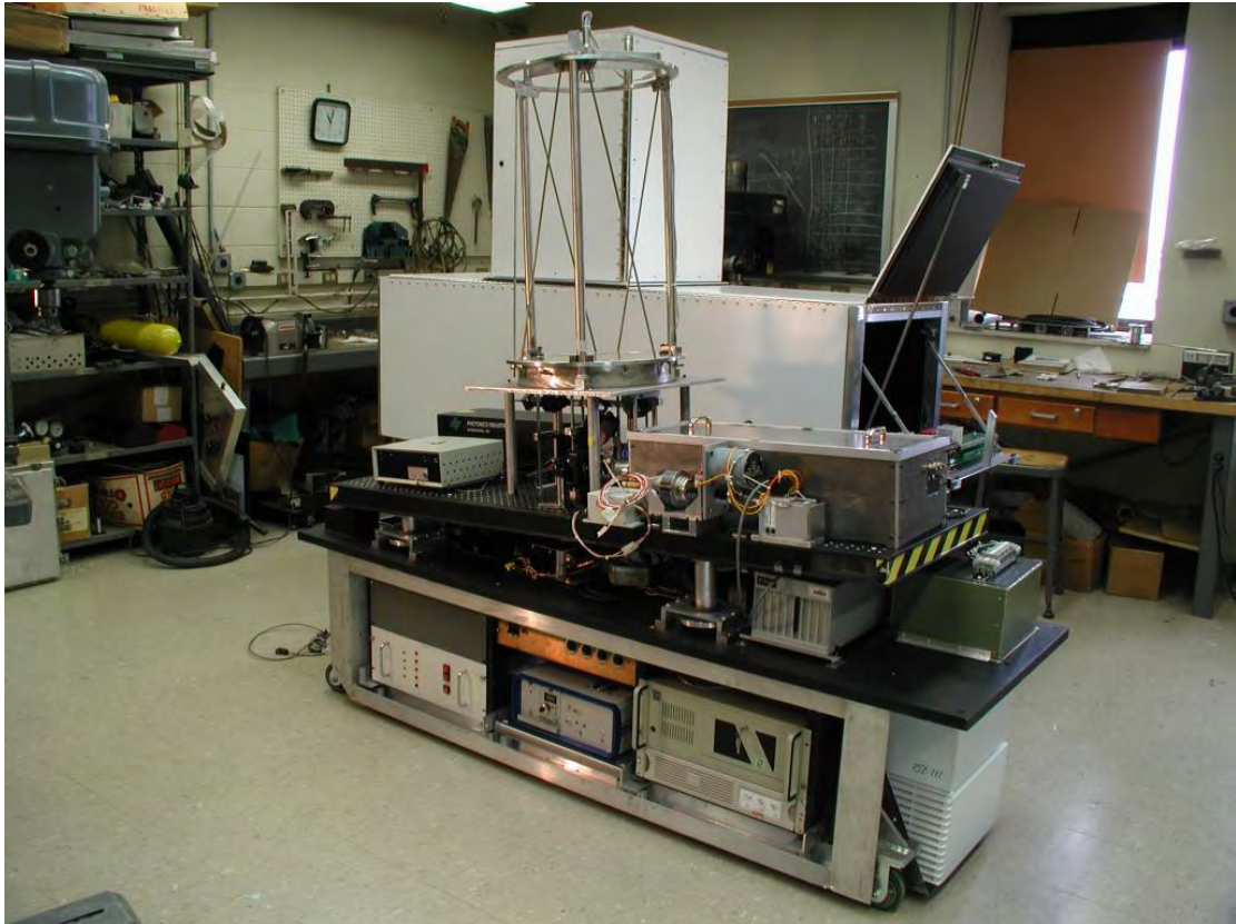
Figure 2.5 – The AHSRL with the protective housing removed. The power supply, laser cooling system, and on-board computer can be seen in the lower compartment. The tilted table is meant to reduce specular reflections due to horizontal ice particles sometimes present in clouds. Among other components located on the table is the laser (the black box on the furthest corner of the table), the primary telescope, and the grey detector box (located at the near corner of the table). The system is temperature controlled and is able to run months at a time controlled only through a network connection.
