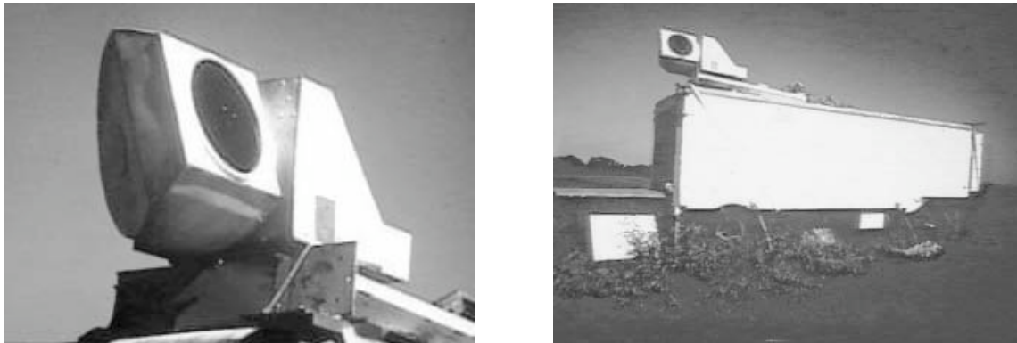
Figure 2.1: The VIL's beam steering unit (left) and the system assembled inside of the semi-trailer (right) with the beam steering unit visible on the roof.
