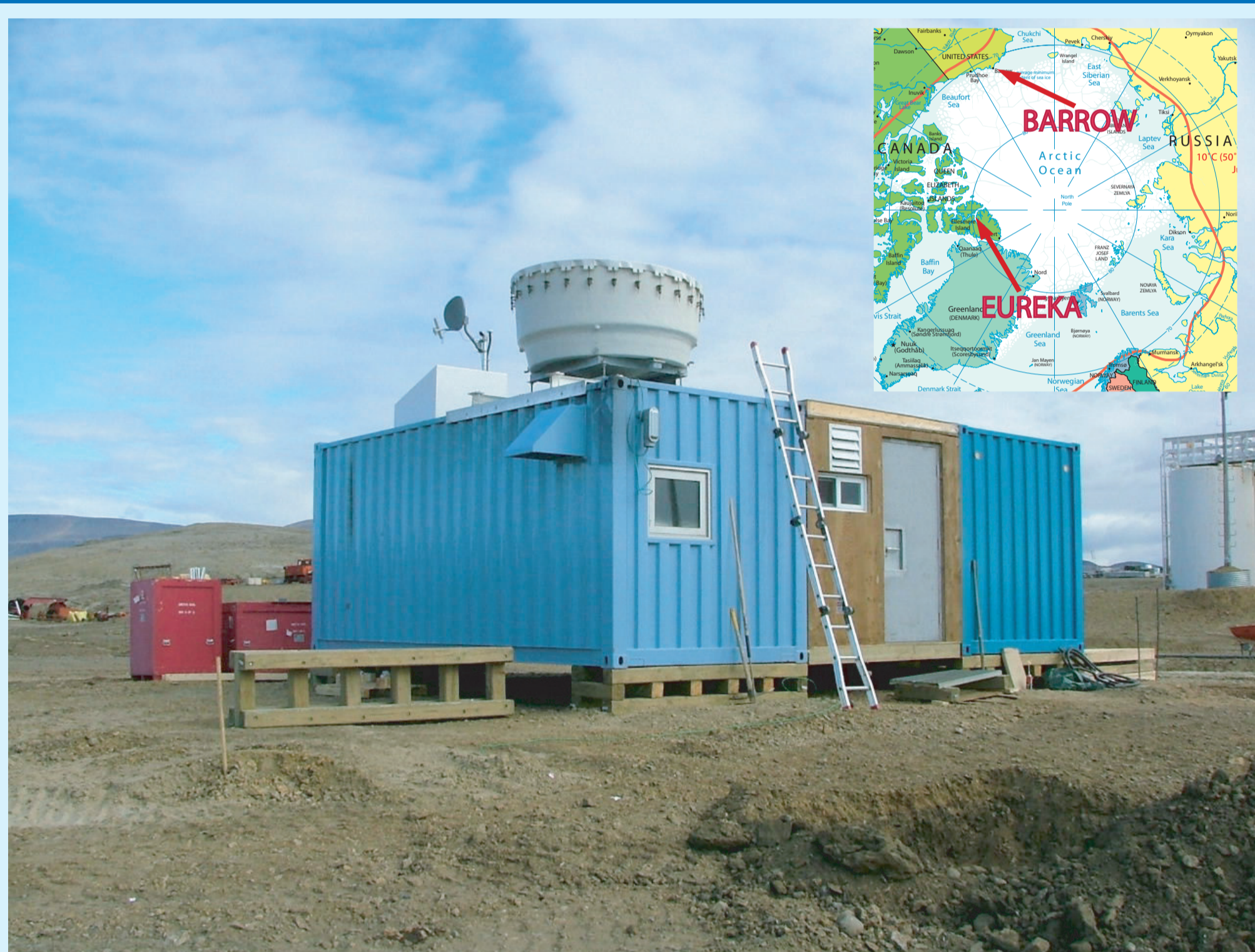
The modified sea-tainer housing the AHSRL together with the NOAA MMCR in Eureka, Canada. The instruments have recorded 10 months of nearly continual data.
