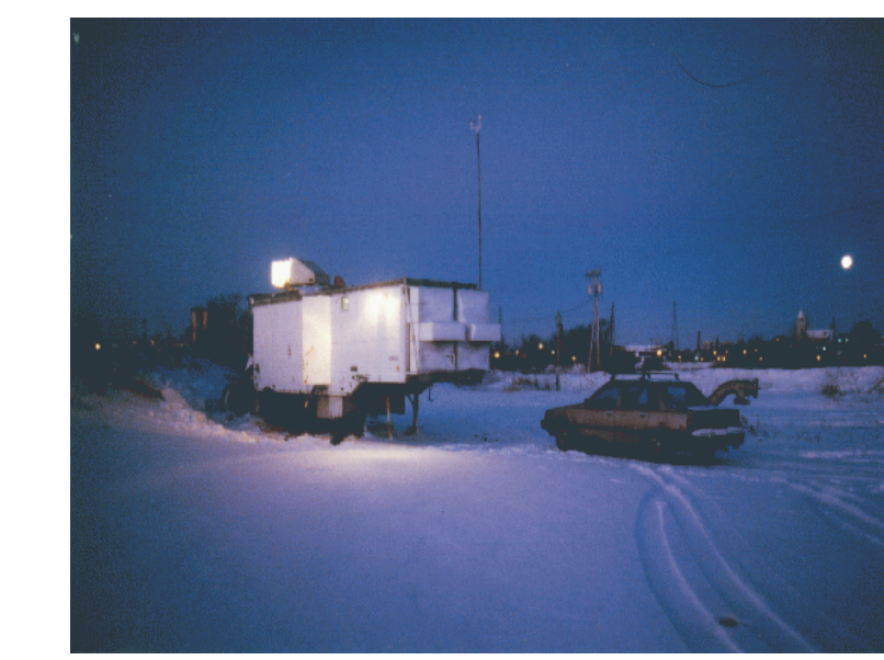
The VIL in Sheboygan, WI during LAKE-ICE. This was taken looking west before dawn. The bright light on the beam steering unit was used to prevent frost formation.
